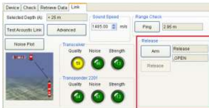
Figure 7-4 – Arming the Release Mechanism
