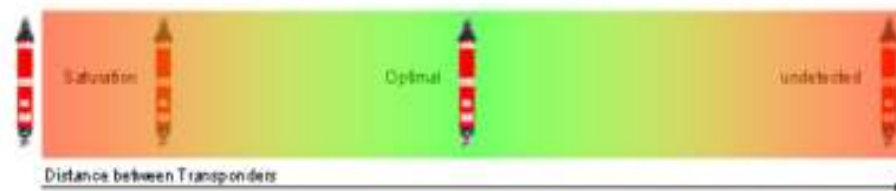
Figure 4-18 – Distance between Transponders
