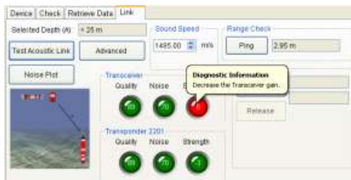
Figure 7-3 – Suggestions to improve acoustic link
