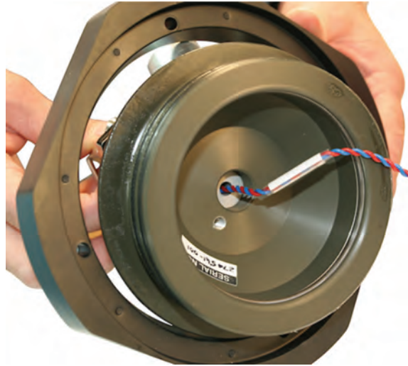
Figure 7-44 – Inspect the Transducer End-Cap
