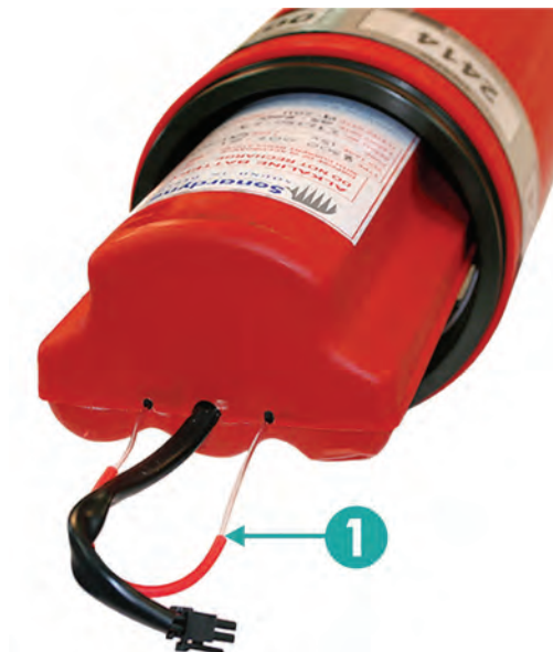
Figure 7-24 – Remove the Battery Pack
