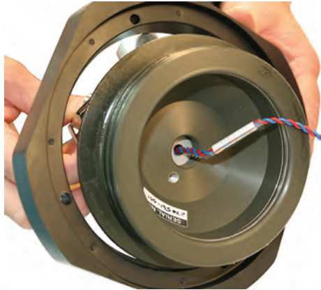
Figure 7-20 – Inspecting the Transducer End-Cap
