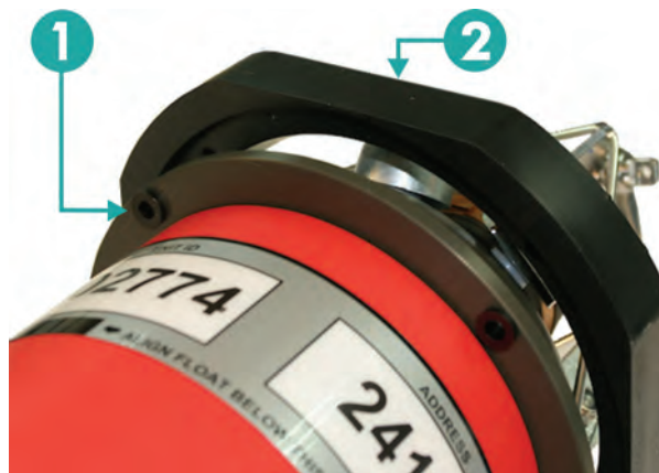
Figure 7-12 – Fitment of Clamp Rings and Bumper Stop
