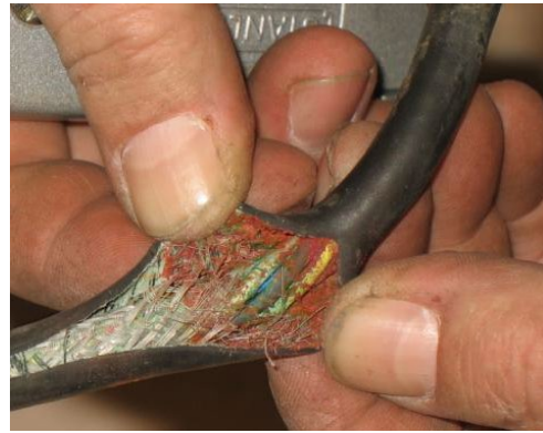
Figure 13. Do not use Zip-Ties Directly on Cables
