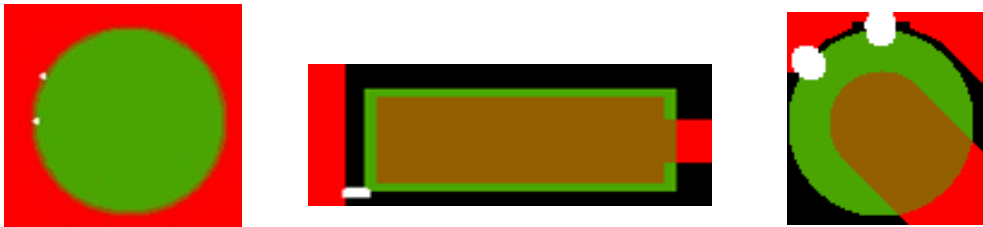
CAM snapshot showing solder mask coverage (copper exposure)
