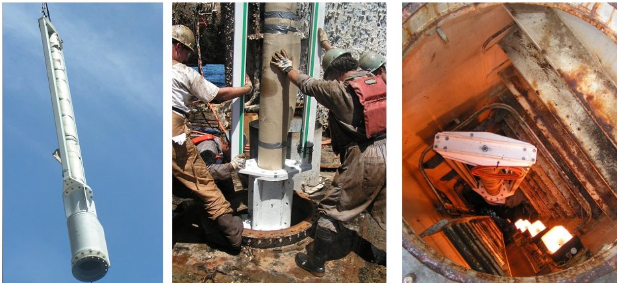
Figure C-2 Through-Hull Mounting (Type 7950 Deployment Machine)
