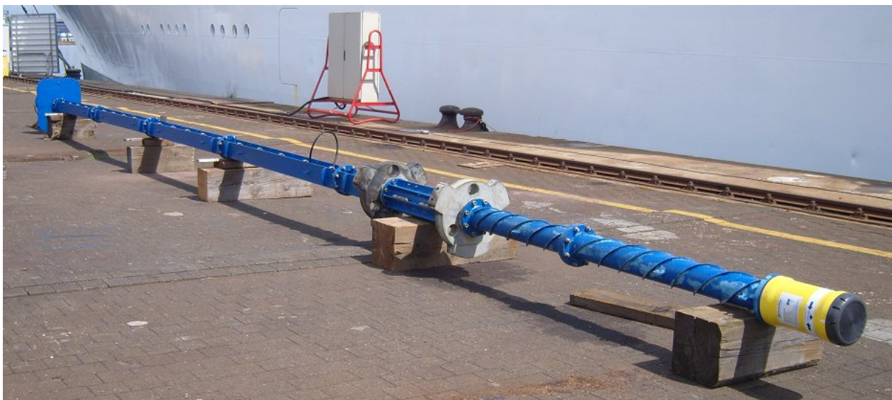
Figure C-4 Through-Tube Mounting (Type 8169)
