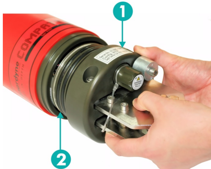
Figure 8-16 Removing the Sensor Endcap
