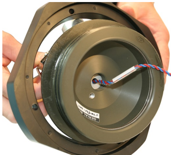
Figure 8–2 Inspecting the Transducer Endcap
