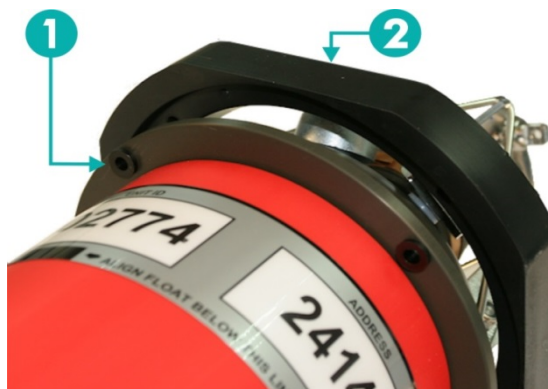
Figure 8–13 Fitting Clamp Rings and Bumper Stop
