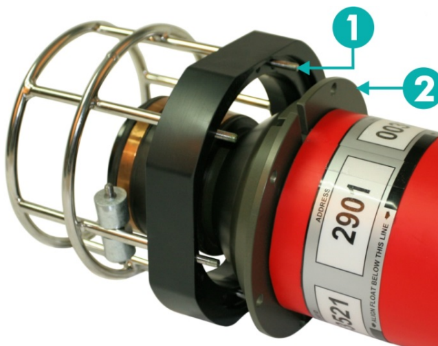
Figure 8-7 Refitting the Guard and Bump Stop
