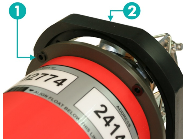
Figure 8-10 Removing the Rubber Bump Stop
