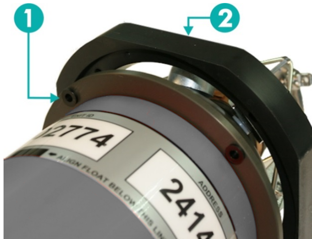
Figure 8–10 Removing the Rubber Bump Stop
