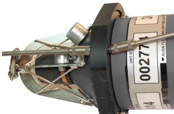
Figure 8-14 Securing Bump Stop to Clamp Rings
