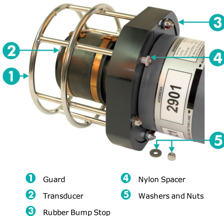
Figure 8-8 Securing the Bump Stop and Guard
