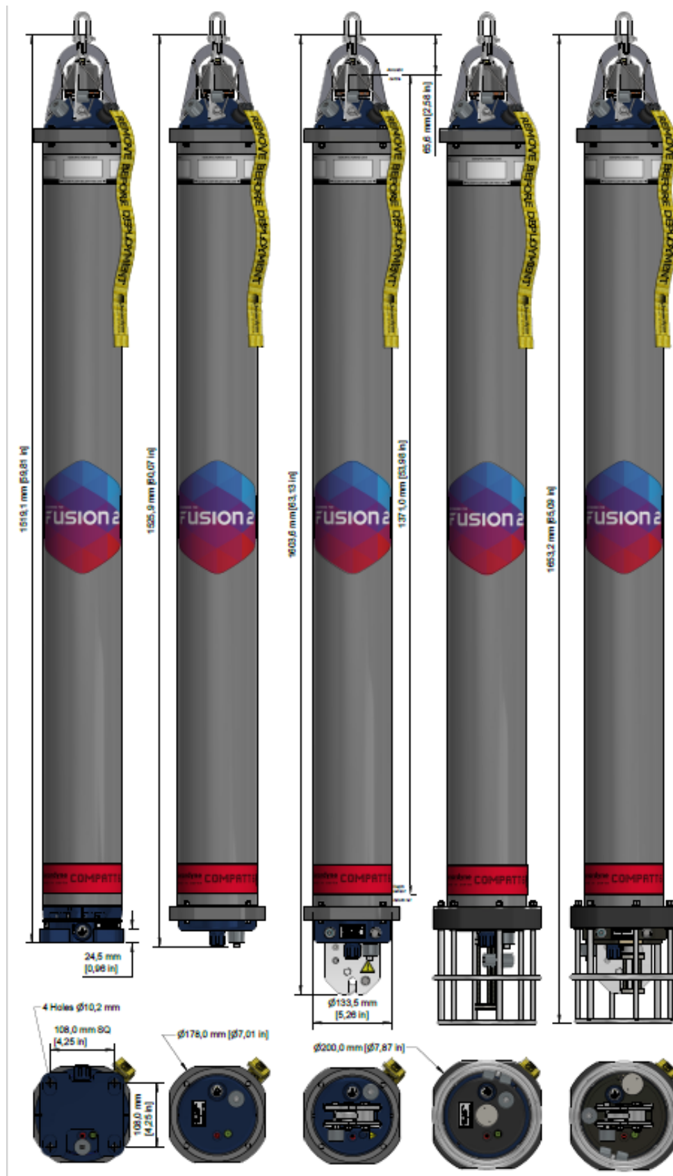
Figure 13–6 Type 830x-3121 (Maxi 3,000 m MF Omni-Directional)
