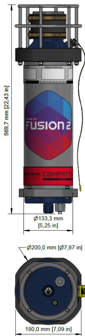
Figure 13–11 Type 830x-3133 (Mini 3,000 m MF Directional)
