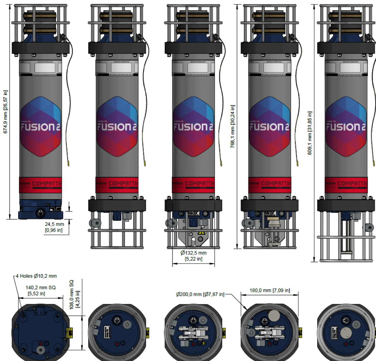
Figure 13–12 Type 830x-3143 (Midi 3,000 m MF Directional)
