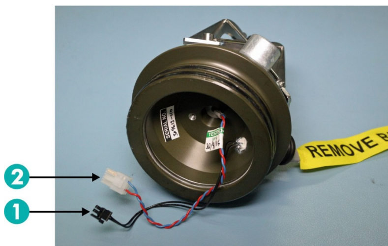
Figure 3–2 Transducer Endcap Internal Connectors
