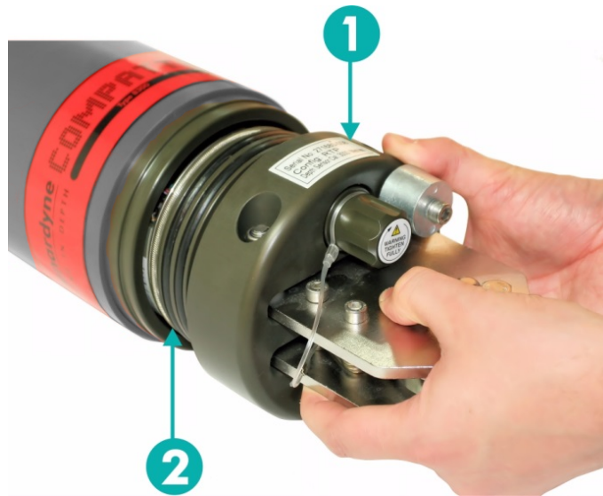
Figure 8-16 Removing the Sensor Endcap
