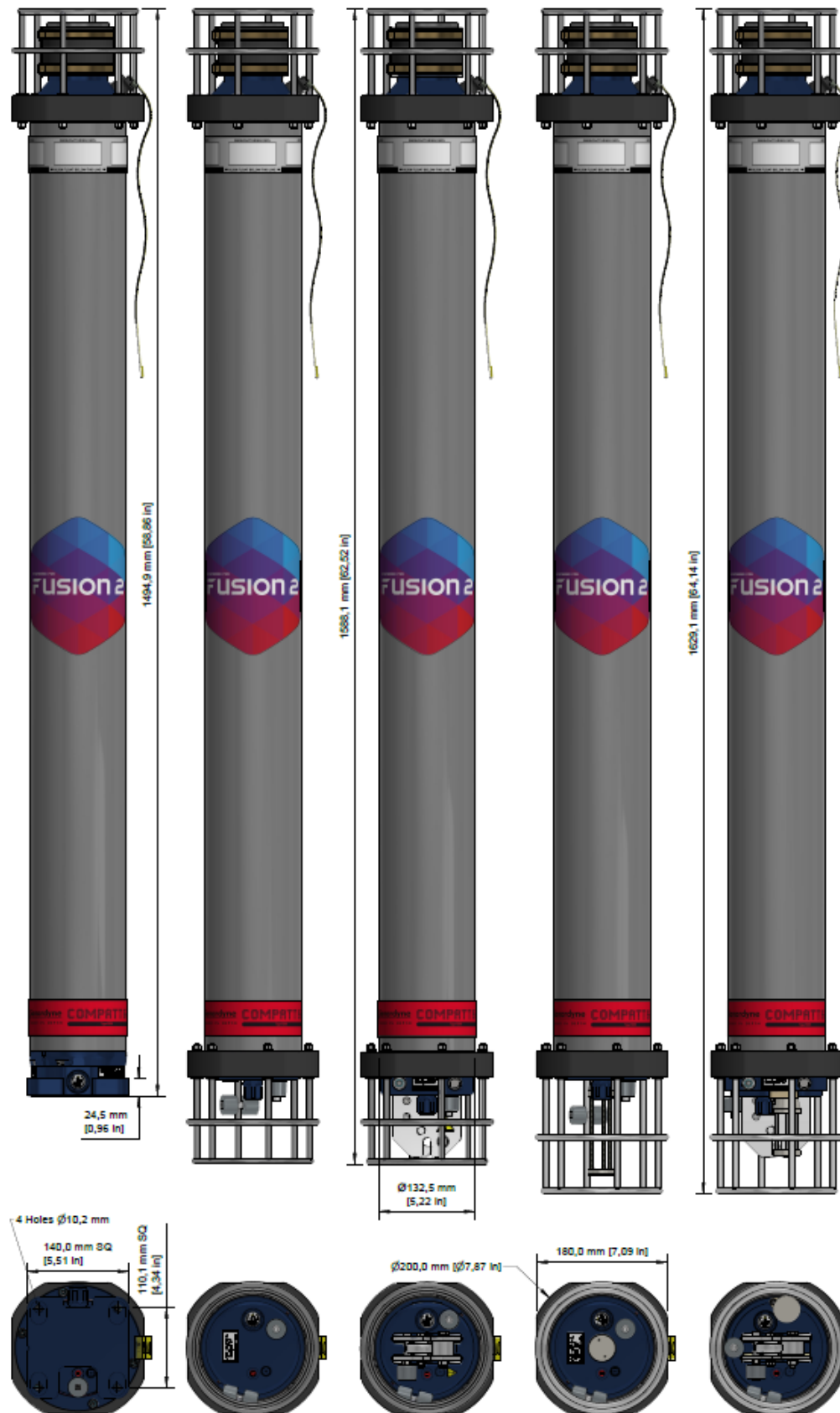
Figure 13–10 Type 830x-3123 (Maxi 3,000 m MF Directional)
