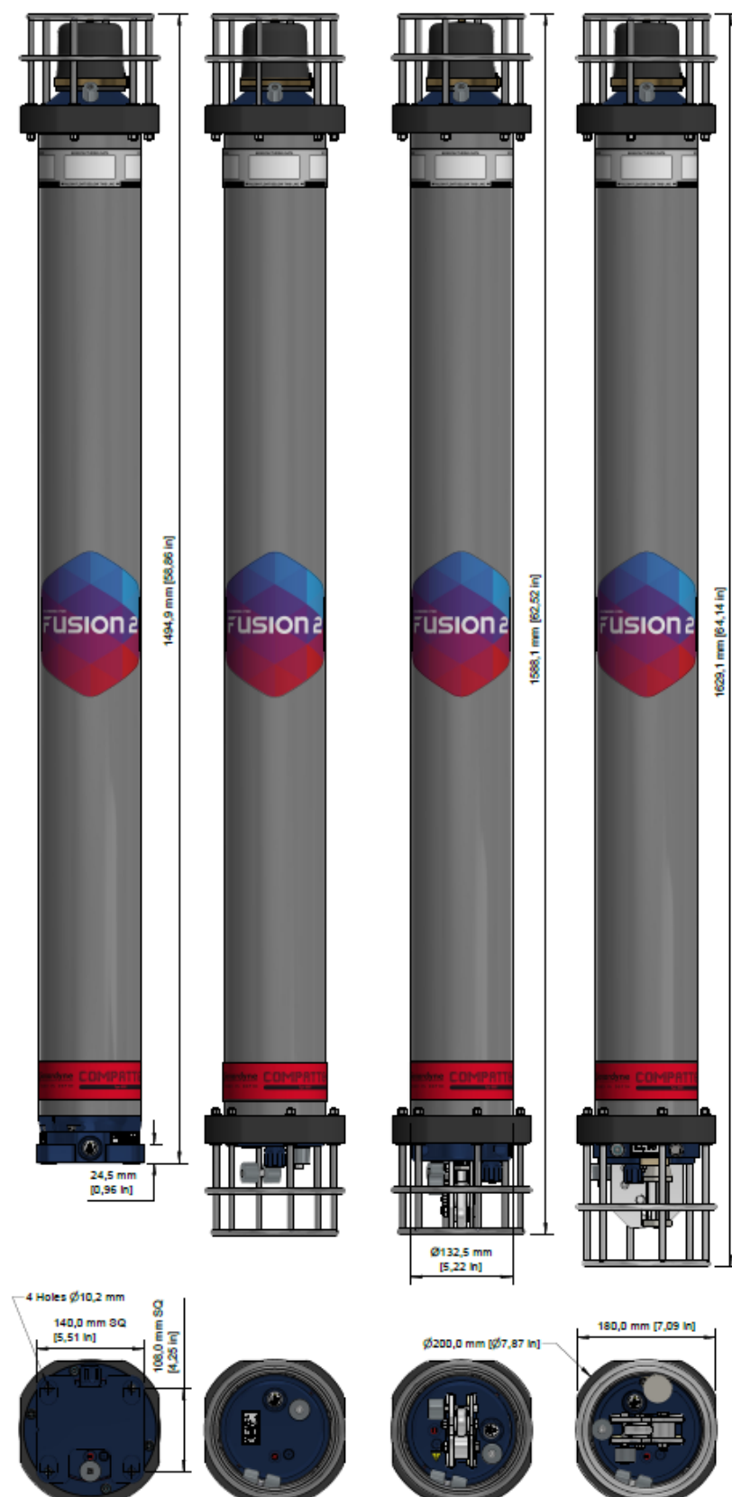
Figure 13–14 Type 830x-3125 (Maxi 3,000 m LMF Omni-Directional)
