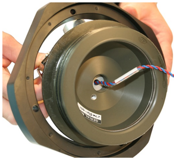
Figure 8–2 Inspecting the Transducer Endcap
