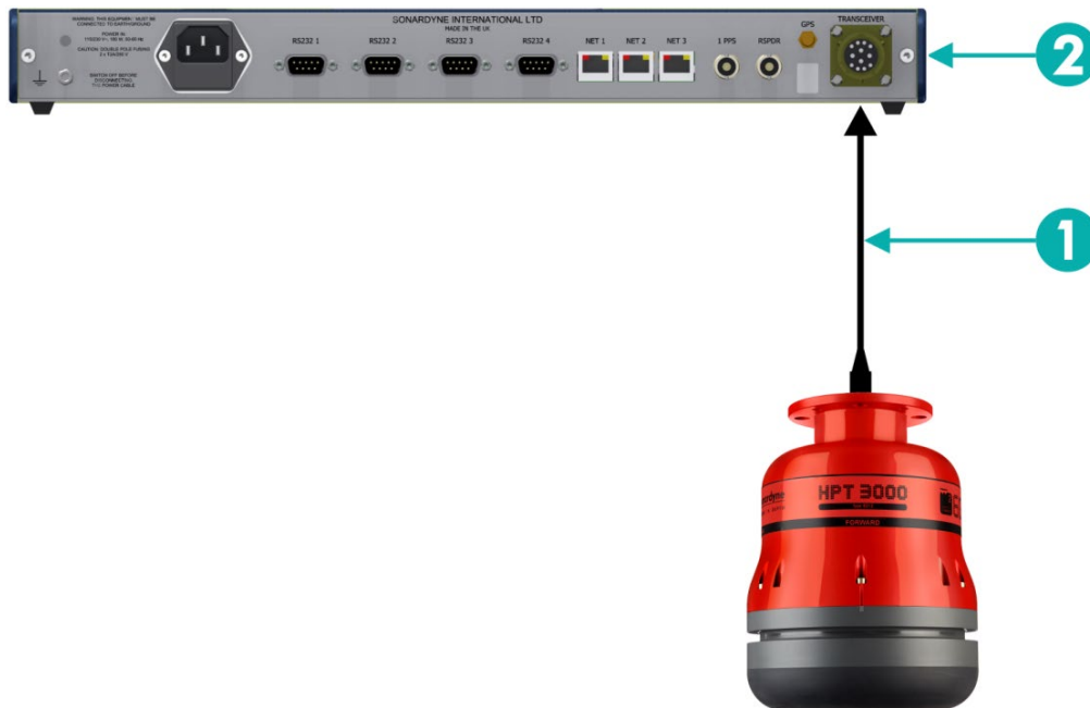
Figure 4-12 Type 8221/8212 USBL Transceiver Interconnections
