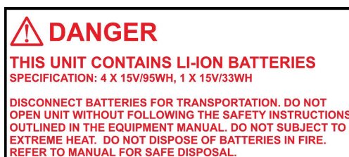
Figure 4-2 – Example of a Lithium-ion Identification Label
