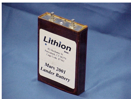
Lithion products Inc. 35 Ah Lithium Ion Cell
