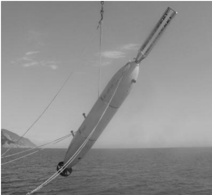
Fig. 2. Caribou the MIT Department of Ocean Engineering’s AUV being launched in the GOATS 2002 Experiment near Italy. The “prong” structure at the front of the vehicle is a Synthetic Aperture Sonar (SAS).
