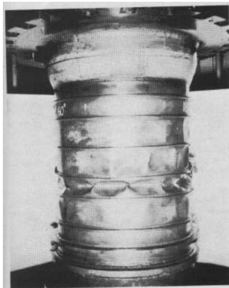
Failure by buckling of shell
