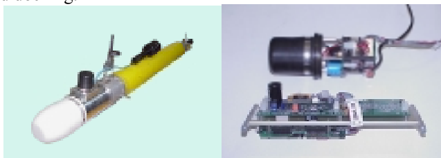
Fig.6 : Taipan with the acoustic modem transducer (length: 1.8m, diameter: 15 cm, weight: 30 kg)
