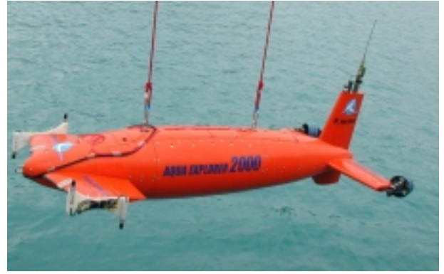
Fig.5 The photograph of AE2000 Four hydrophones of the passive sonar are mounted at the end of the fore-wing
