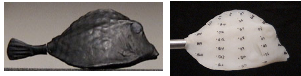
Fig. 2. Models constructed using stereolithographic rapid-prototyping. The model on the left was used in digital particle image velocimetry and force experiments. The model on the right was used in pressure experiments.
