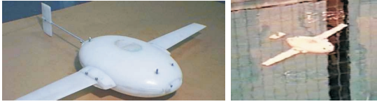
Figure 1.1: Experimental, laboratory-scale underwater glider ROGUE.
