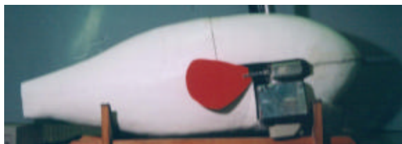
Fig.2-3 Fish robot "BASS-II" equipped with a pair of 2MDMPFs
