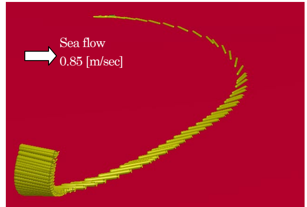
Fig. 6 3D-View of Vertical Ascent Motion in the case of No Thruster Failure
