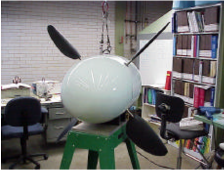
Figure 1 - Pilotfish. The Pilotfish was constructed by Nekton Research, LLC. It uses four flap propulsors to propel itself through the water and is remotely operated by an outside user. The Pilotfish has excellent acceleration and deceleration capabilities, as it is capable of coming to a complete stop from full speed in a tenth of its body length.
