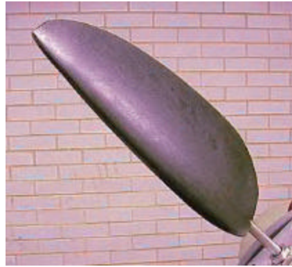
Figure 2 - Fin Flap Propulsor. Shown here is one of the fin flap propulsors mounted on the side of the Pilotfish. The fin is constructed of a polyurethane elastomer and was cast by Nekton Research, LLC.
