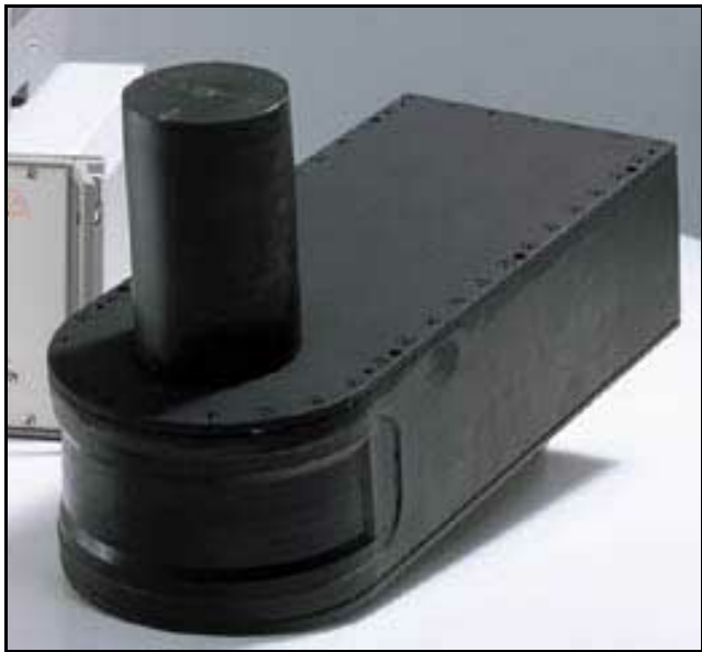
Figure 4.2. The SeaBat 9001 sonar used in both the simulation study and the sea trials.
