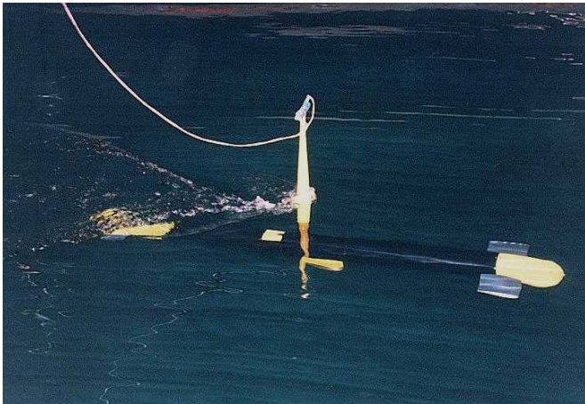
Fig. 5. AMPS 0.29 scale model operating in simulated following seas in the David Taylor Model Basin (DTMB).
