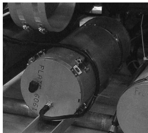
Fig. 10. USNA inertial guidance package mounted on the JHUROV.
