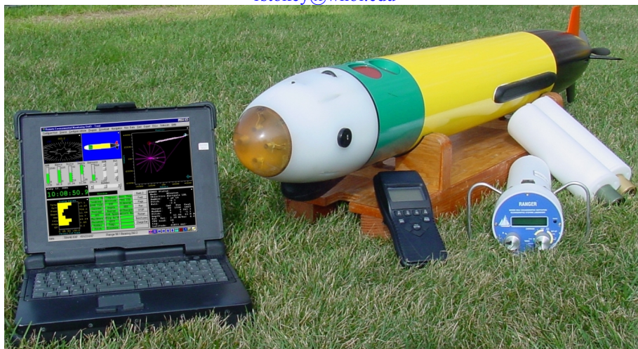
Fig. 1. Laptop, REMUS, GPS receiver, Ranger and Transponders
