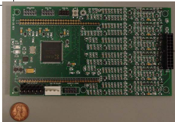
Front side of the 6-channel signal conditioning board
