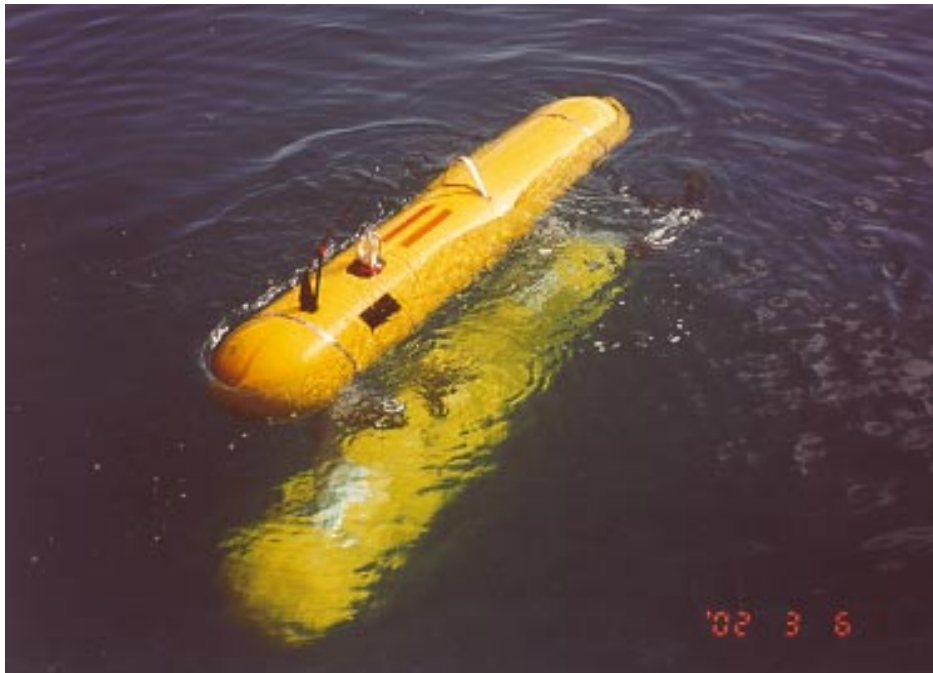
Figure 1. The SeaBED AUV. A hover capable vehicle its suite of sensors include a side-scan sonar, a pencil beam scanning sonar, and a 1280x1024 12 bit CCD camera.
