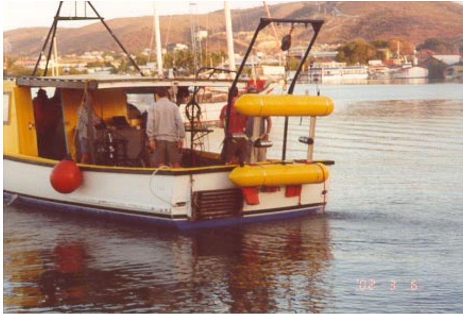
Figure 8. One last image. We can run SeaBED off of very small platforms. This time we could not even get the vehicle on board but had to instead lash it to the stern of the trusty R/V Sultana. OK, so we proved a point (and next time we will be on a UNOLS class vessel) but the fact remains that all we need to support the vehicle is a power supply, a laptop and a navigation transponder.
