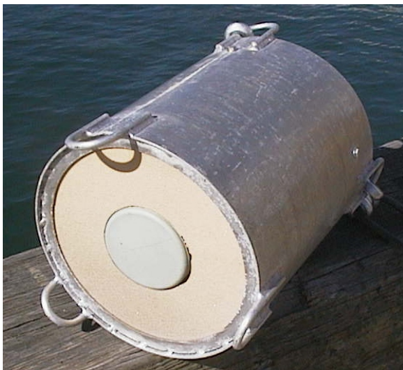
Fig. 2. Directional mass-loaded piston receiver encased in foam baffle to reduce the effects of surface noise and reflections.
