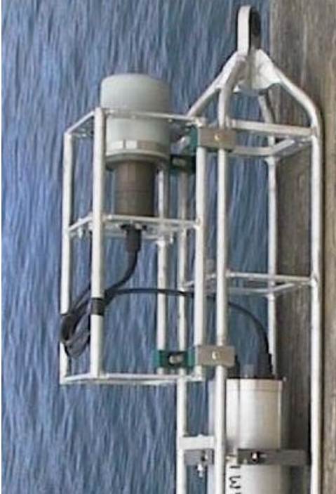
Fig. 1. Transmit electronics in pressure case and directional projector mounted to side.
