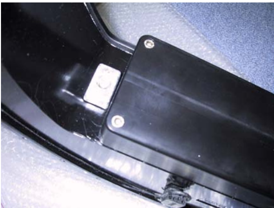
Figure 2b. Pressure Equalization. Bladder is painted to protect against corrosion.
