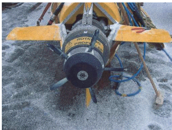
Figure 1. Autosub's five-bladed propeller. The large diameter hub houses the direct-drive DC propulsion motor.
