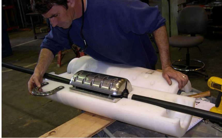
Figure 4. The cable clamp grips tightly around a relief cut into the cable jacket. The white plastic adapter locks with the cable floats at each end of the clamp assembly.
