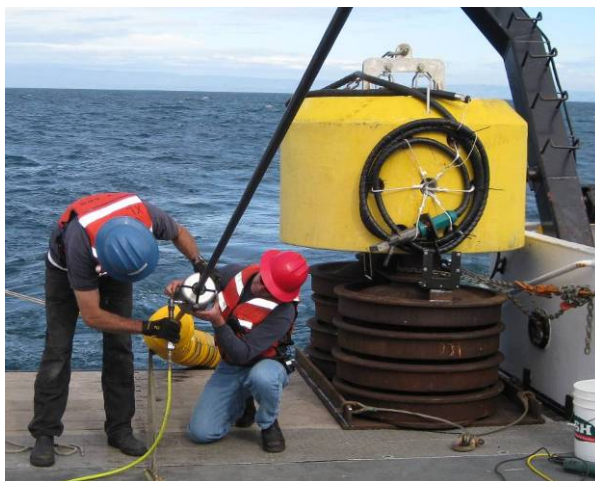
Figure 6. The anchor float and anchor. After launch the anchor float separates from the anchor.
