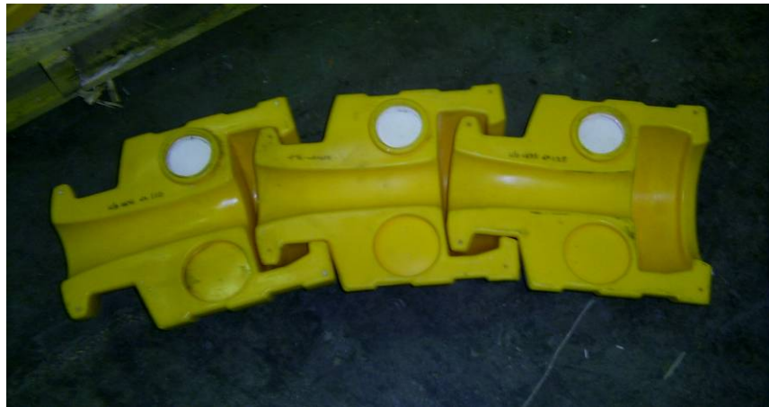
Figure 5. Cable floats before assembly of the two halves illustrating the interlocking design that limits the riser cable bend radius.
