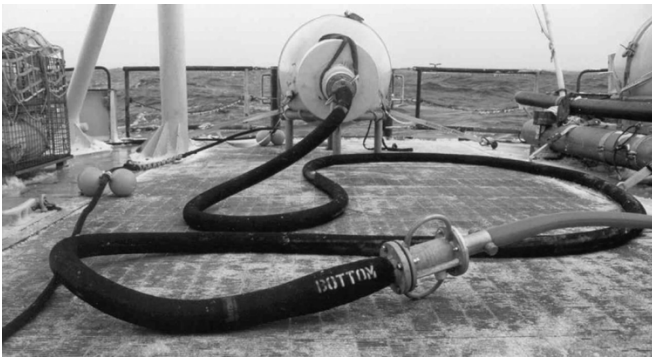
Fig. 2. Snubber hose placed inline between a surface buoy and the top a Vectran EOM mooring cable to increase compliancy of the mooring and decrease dynamic tensions in waves.
