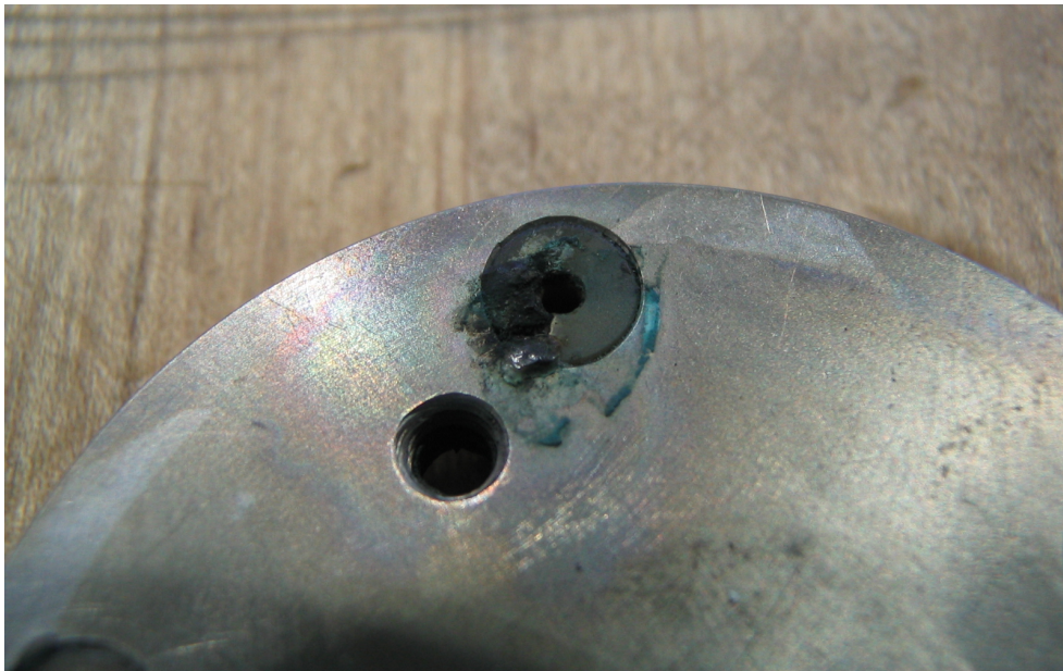
Figure 3. Photograph of internal bulkhead in the failed ODI FITA showing evidence of insulation breakdown, erosion and copper plating. This is the evidence that points to the FITA having failed during powered operation, not after being cut from the non-powered cable assembly during recovery (photo from ODI).
