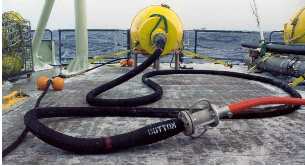
Figure 4. Snubber hose ready for deployment in the Labrador Sea.
