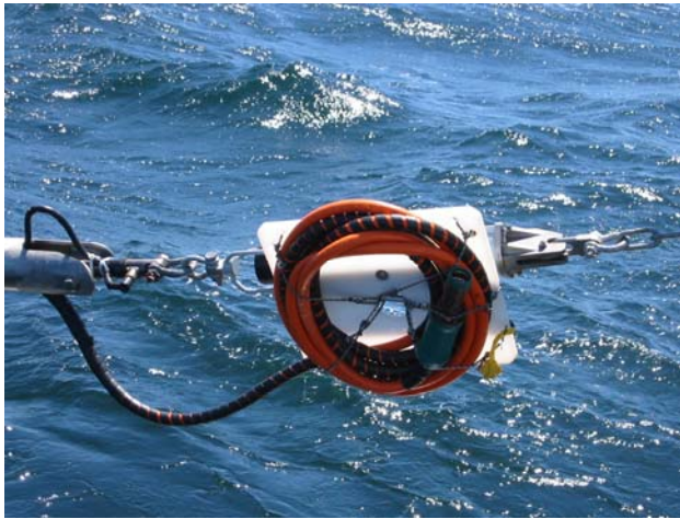
Figure 2. Lower termination and release at the time of deployment.
