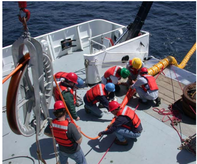
Figure 1. Illustration from deployment showing large radius snatch block.
