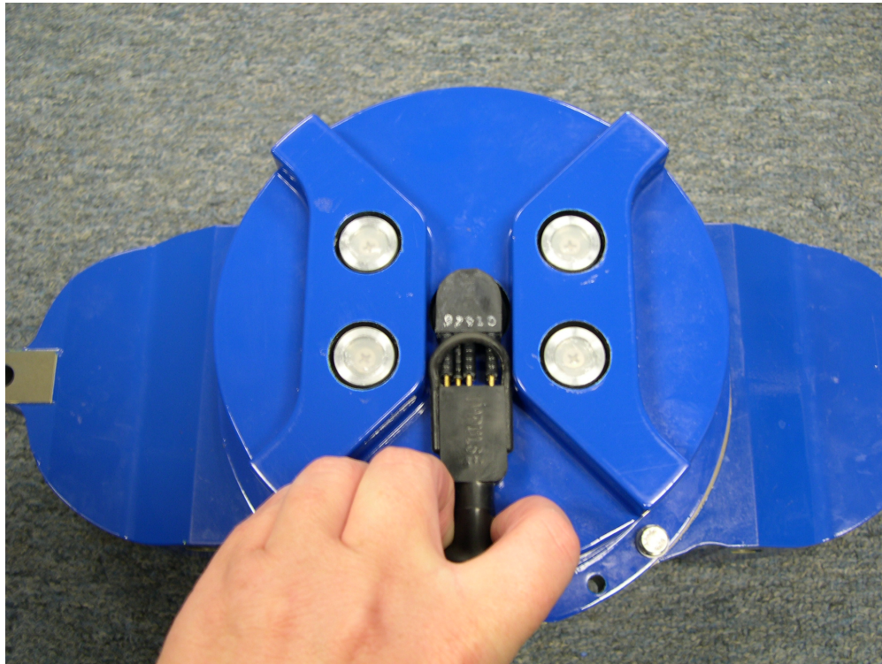
Figure 7. Removing the I/O Cable
