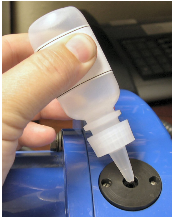
Figure 16. Filling the Pressure Sensor Cavity with Oil
