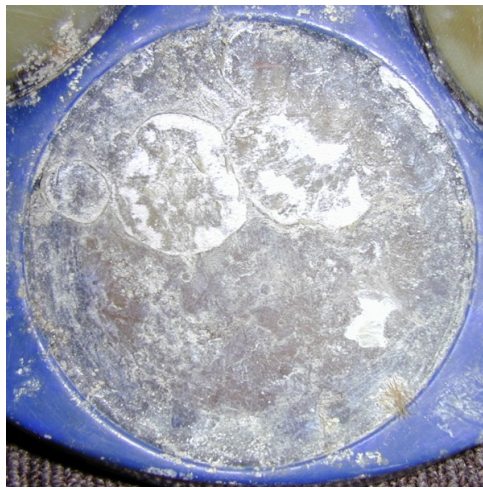
Figure 6. Barnacle Damage to Urethane Face
