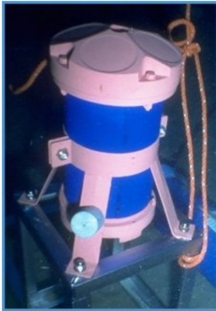
Figure 15. Antifouling Paint Applied to a WorkHorse Sentinel
