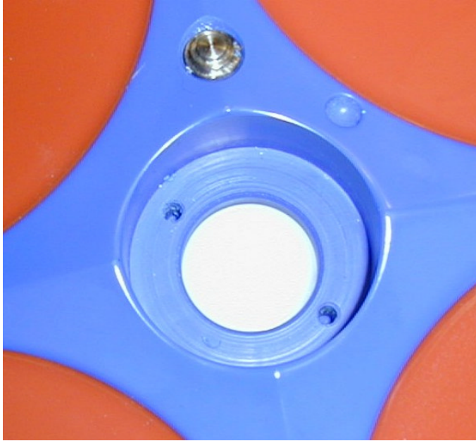
Figure 3. View of Pressure Sensor/Insert Plug with Cover Plate Removed
