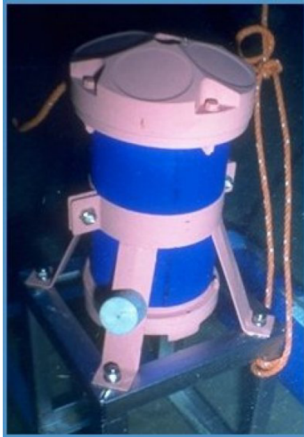
Figure 10. Antifouling Paint Applied to a WorkHorse Sentinel
