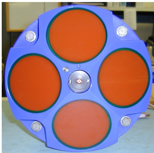
Figure 1. WorkHorse Transducer Face View
