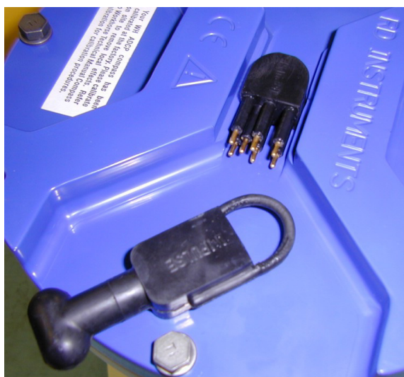
Figure 2. WorkHorse End-Cap Connector View
