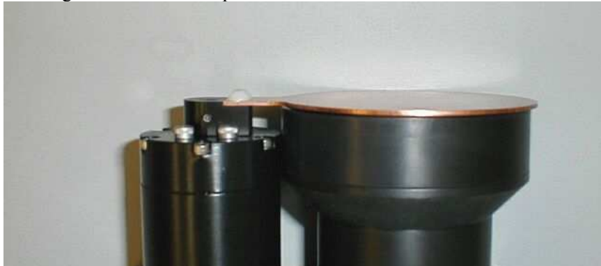
Figure D-4: Shutter/Sensor gap
