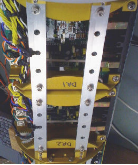
Power Can photo --- Coupler board mounts to these rails with components underneath
