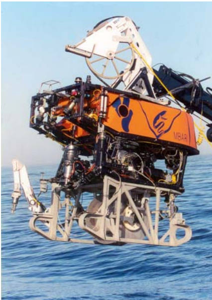
Figure 16: Cable laying toolsled on ROV Ventana
