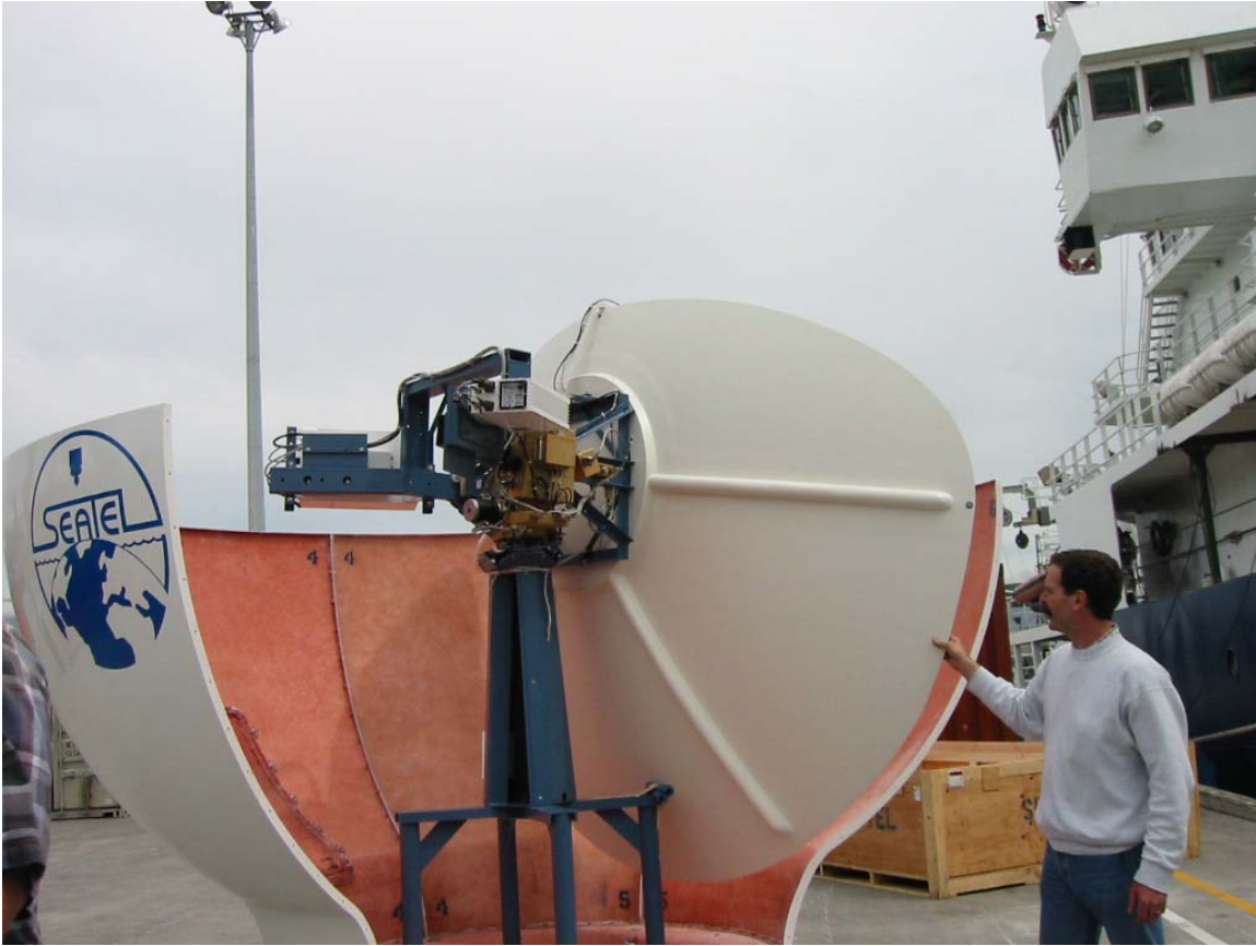
Figure 19: The SeaTel Antenna with the radome half completed.
