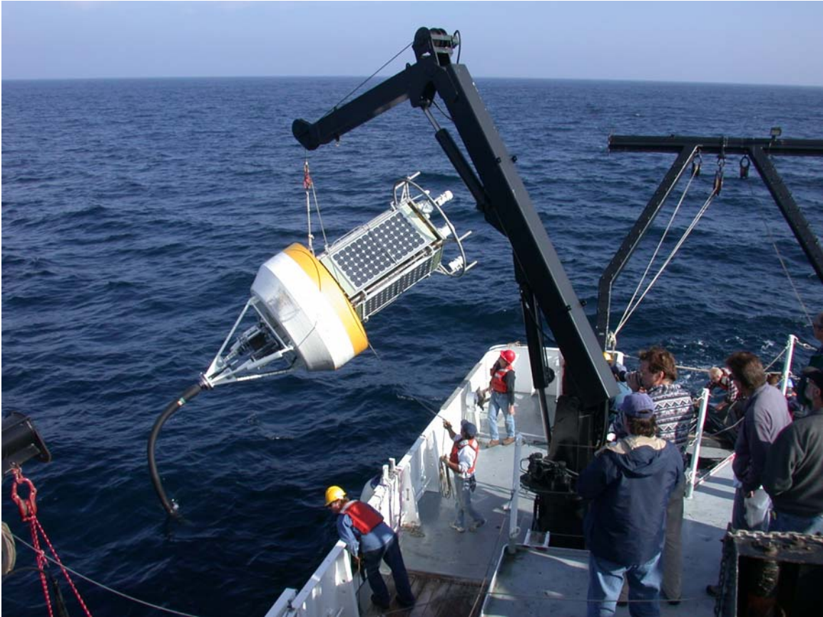
Figure 11: Deployment of MOOS mooring off the back of the Point Sur
