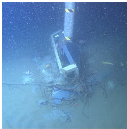
Figure 2 - After: Revisited RIN "site" after 30 days: RIN moved 170m down canyon and was partly buried. Note battery cage wrapped around masts. Another RIN deployed nearby was never found. There was no obvious triggering event.
