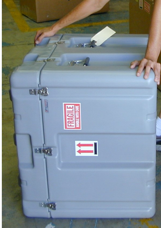
Figure 9. Rotating the ADCP/Shipping Case During Compass Calibration
