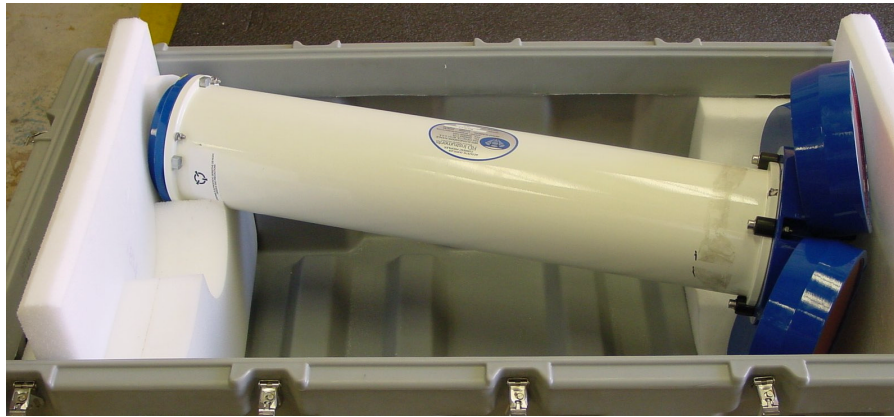
Figure 11. Self-Contained Long Ranger Tilted Position in Shipping Case
