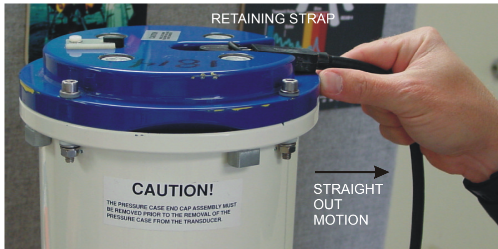
Figure 2. Connecting and Disconnecting the I/O Cable
