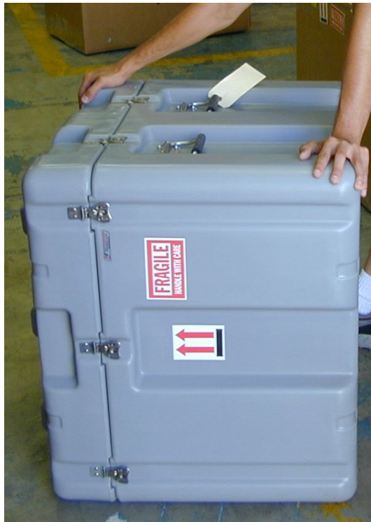
Figure 13. Rotating the ADCP/Shipping Case During Compass Calibration
