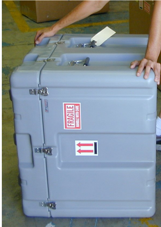
Figure 9. Rotating the ADCP/Shipping Case During Compass Calibration
