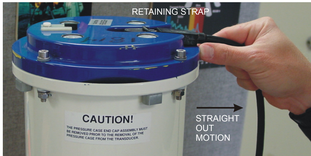
Figure 2. Connecting and Disconnecting the I/O Cable
