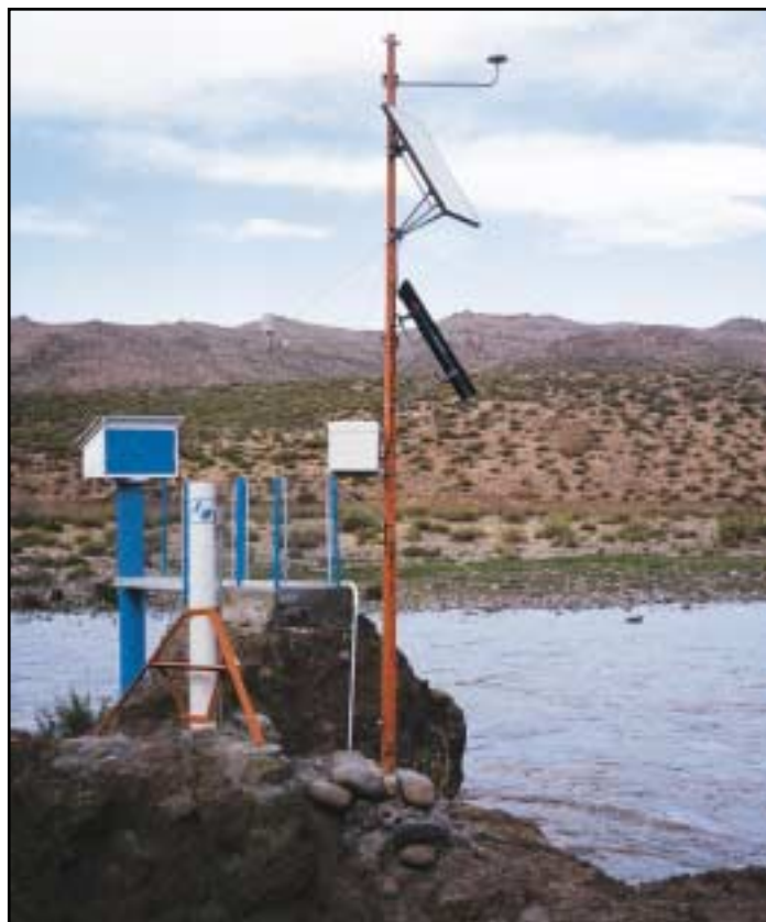
The INMARSAT-C satellite system provides telecommunications for remote Argentine stations where phone lines are impractical.
