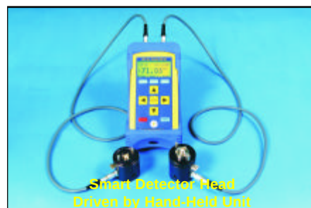
Smart Detector Head Optical Power Meter and Interchangeable Receptacles
