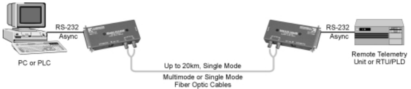
Typical RS-232 asynchronous application using TC1000s
