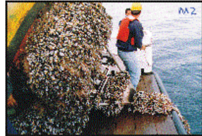
Figure 1. Biofouling on the M2 mooring, the number one problem for the moorings. The moorings are pulled in on a regular basis for maintenance: rebuild, cleaning and replacing instruments. Routine maintenance is also done in situ, with technicians boarding the mooring while out at sea.
