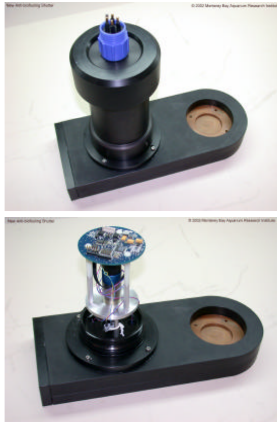
Figures 3a & 3b. a.) The shutter is a watertight housing composed of a base with a copper plate that opens and closes over an instrument's optical window. b.) Within the watertight housing, an embedded controller triggers a motor with a shaft encoder to drive the copper plate open and closed.
