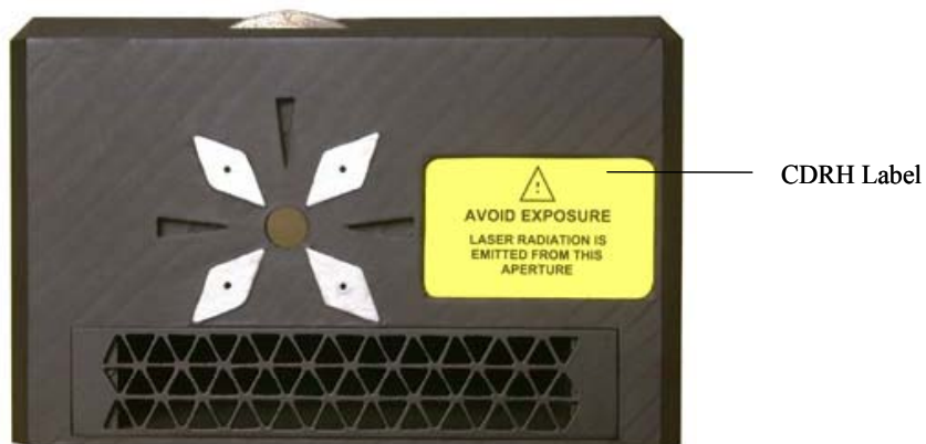
Figure 1.1 Front-end view of Invictus 785 nm laser showing location of CDRH compliance labels.
