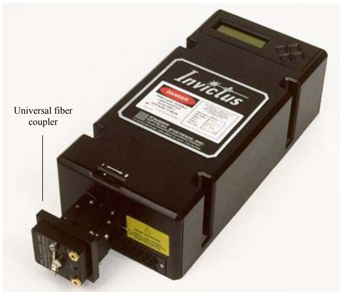
Figure D.1 Invictus 785 nm laser showing location of the universal fiber coupler.
